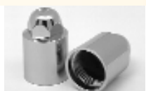
P/N 000080 Chrome plated ABS nut cover 1.669" height 3/4" hex, fits 006XXX
